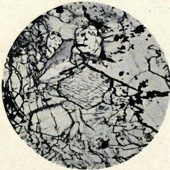
4.—Glaucophane, trans. sect. Ord. L. Showing form and cleavages.
